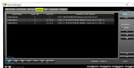
7. Click the tab of "DMX devices", set port status to "ON" if connected successfully. Now, you can use computer to control lamps via ArtNet-DMX-8.
